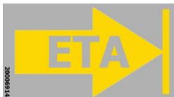
Return air from building ( ExTract Air )
